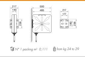
THE HOSE REELS ARE EQUIPPED WITH A UNIVERSAL HOSE STOP; THOSE WITH HOSE ARE PROVIDED WITH A 0,6 M INLET CONNECTION HOSE.
